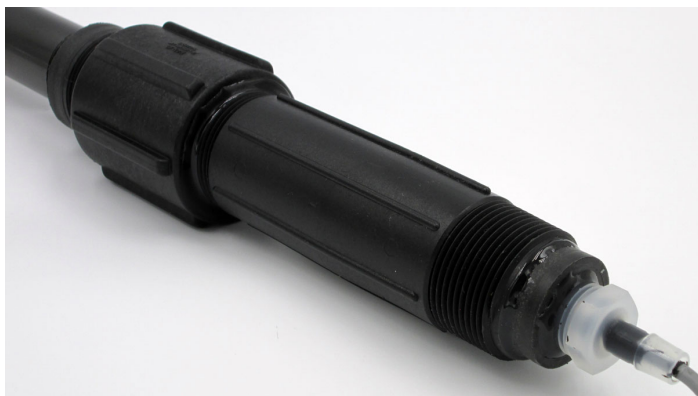
Detail rear view close-up of self-powered sensor assembly. The 1.25” MNPT threads are interface with 1.25” FNPT threads on standpipe or immersion rod for submersible installations with hose to be fitted onto the 3/8” hose barb.
