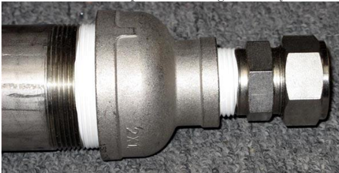
2"X1" Reducer Coupling (Provides Blowout Protection) and 1" Compression Fitting Assembly
