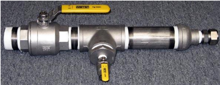
2"X1" Reducer Coupling (Provides Blowout Protection) and 1" Compression Fitting Assembly
