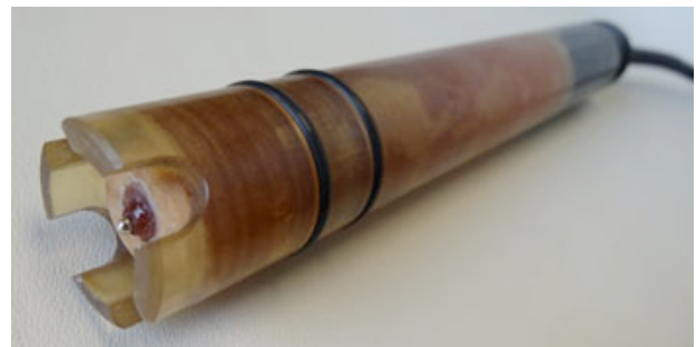
Close-up of 5831 sanitary ORP sensor with “GR” Tines & O-rings installed
