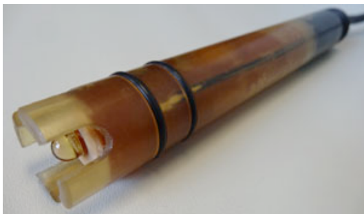
Close-up of 5X31 sanitary pH sensor with “GR” Tines & O-rings installed
