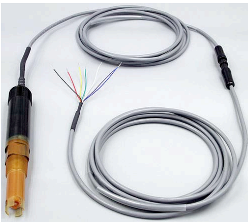
6X31 RADEL-KYNAR series pH sensor with integral preamplifier and Q7M quick disconnect snap connector interfaced with mating Q7F to tinned leads extension cable. The Q7M/Q7F connector system is rated NEMA 6P when interfaced and suitable for rugged field use.
