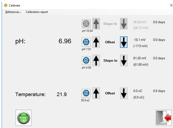
**Step 1** - Perform the pH buffer “Offset” calibration near pH7
