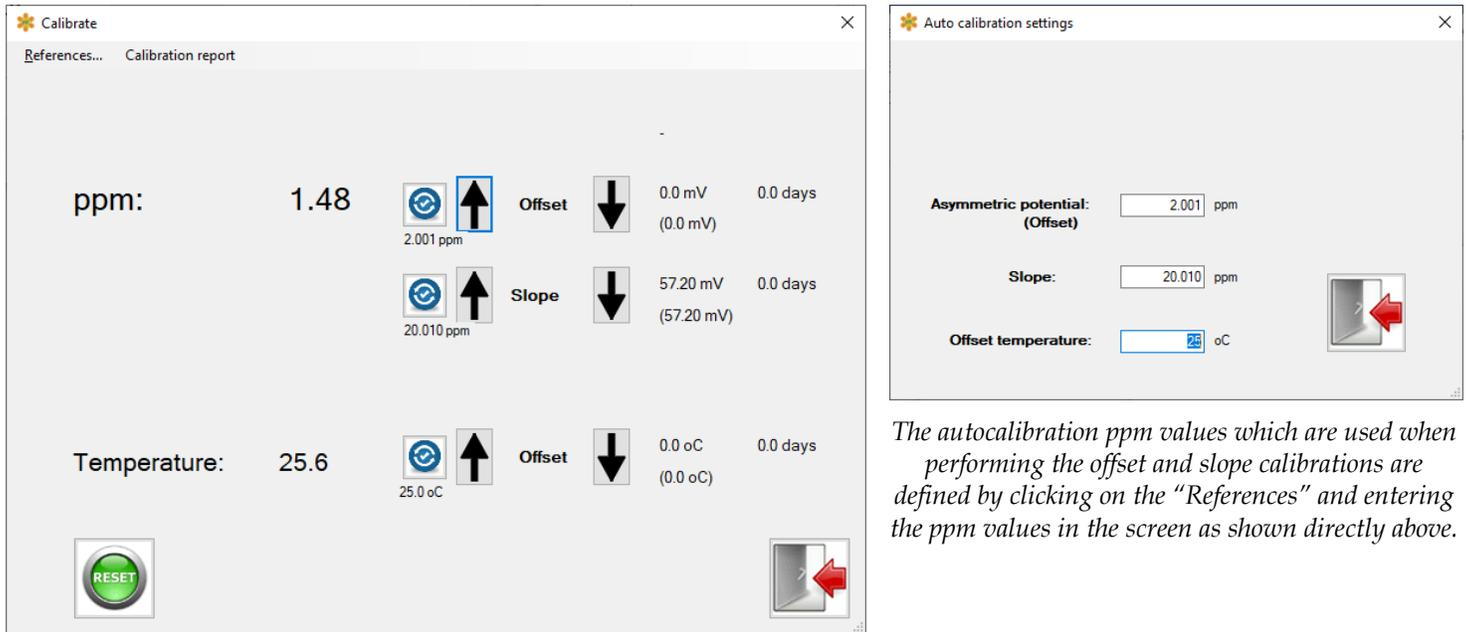
The screenshot displays two windows from the IOTRON™ software. The 'Calibrate' window shows a ppm reading of 1.48 and a temperature of 25.6. It includes calibration controls for Offset (0.0 mV), Slope (57.20 mV), and another Offset (0.0 oC). The 'Auto calibration settings' window shows 'Asymmetric potential (Offset)' set to 2.001 ppm, 'Slope' set to 20.010 ppm, and 'Offset temperature' set to 25 oC. A red arrow points to a 'References' button in the settings window.
