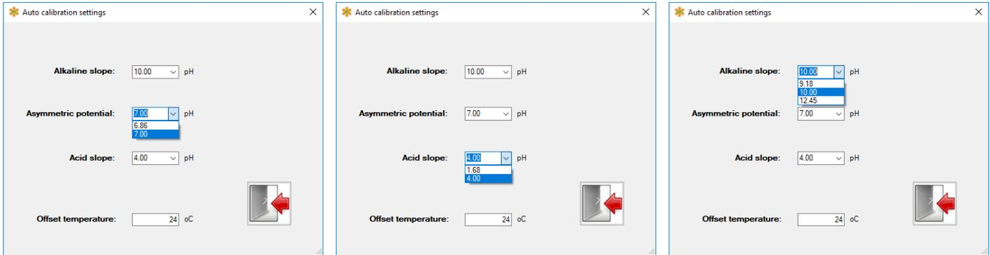
The reference temperature value is not selected from a drop down but rather is entered into the appropriate field.
