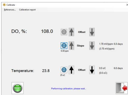
When autoread calibration is initiated, “Performing calibration, please wait...” shown while stability test is performed.
