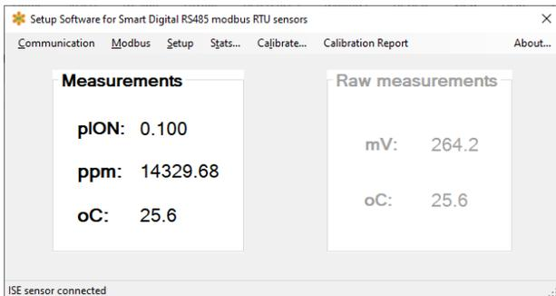
*A 0.1mV change in the ISE sensor always produces a systematic corresponding response in pION units. In contrast, the same 0.1mV change in the ion selective sensor reading produces a non-linear response in ppm.*
