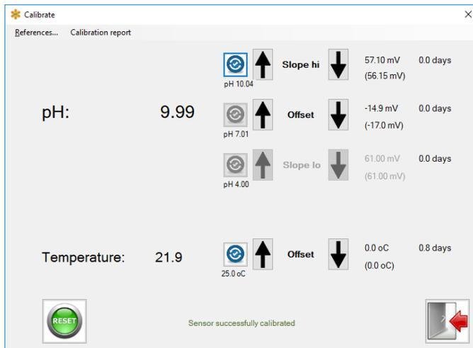
**Step 3** – Perform “Slope Hi” calibration in the alkaline range
