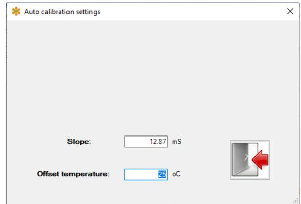
*The autocalibration conductivity values are used when performing the slope lo and slope hi calibrations and are defined by clicking on the “References” and entering the mS values in the screen as shown directly above. Click on the “Exit” icon to save the entered values before calibrating.*
