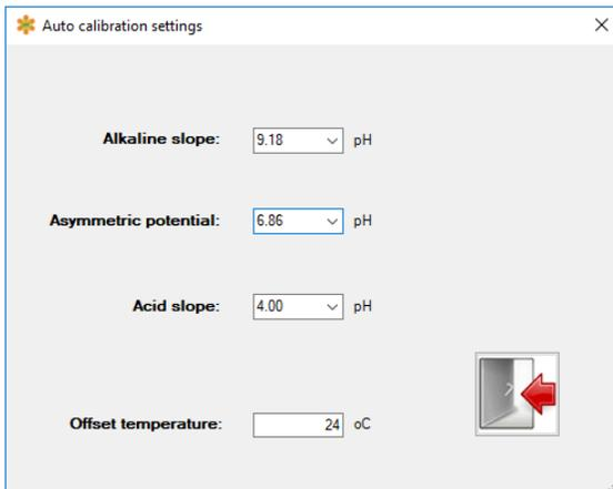
Typical values for most European pH installations are 4.00, 6.86 and 9.18 pH buffers. This is the best practice pH buffer scheme for most pH measurements that do not commonly go much below pH 4.00 and or else much above pH 9.20. The 6.86 & 9.18 pH buffers are most stable than the 7.00 & 10.01 pH buffer counterparts but are still more prone to shifting than the very stable 4.00 pH buffer. Care should be taken that the pH 9.18 buffer is fresh to ensure best alkaline slope calibration results.
