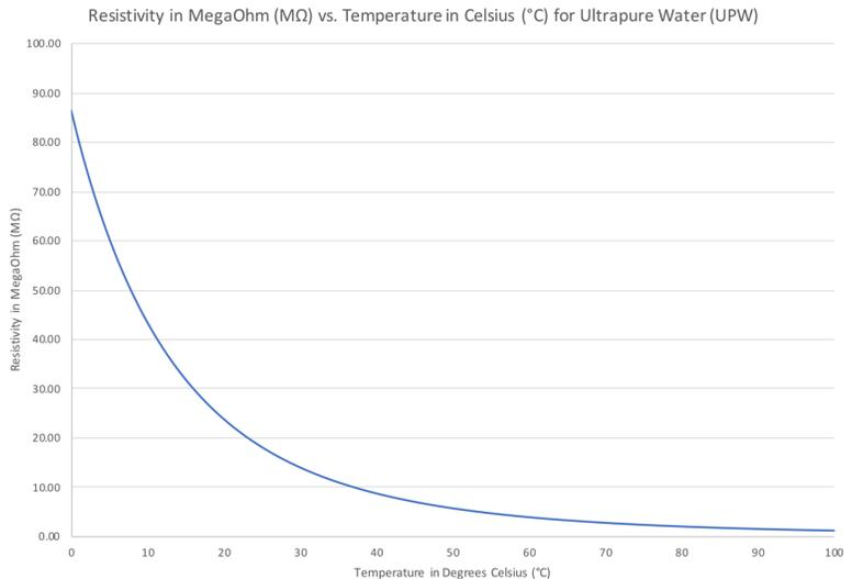
Graph above shows relationship between the resistivity of pure water at various temperatures. Computed resistivity MegaOhm (MΩ) units are the inverse of measured conductivity and so are the mirror image of the conductivity at various temperatures for ultrapure water (UPW). The graph above shows absolute raw resistivity at various temperatures. Resistivity values sent include ATC referencing reading to 25 °C state.
