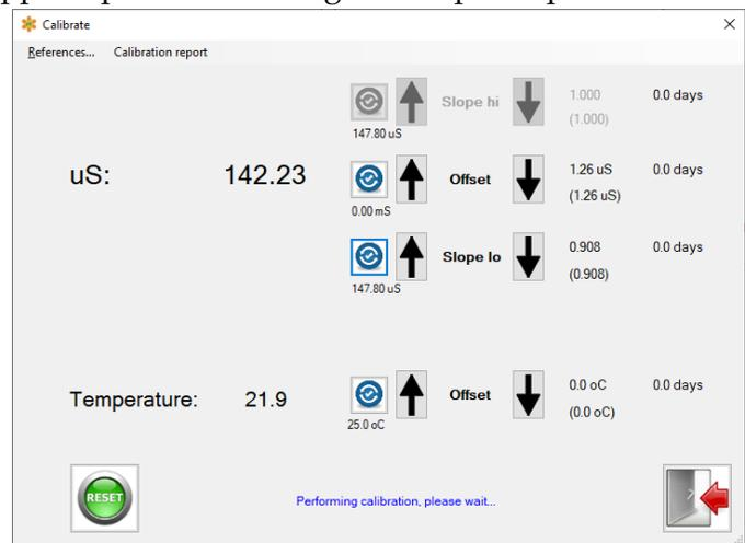
**Step 2 - Perform Slope calibration within range of cell used**
