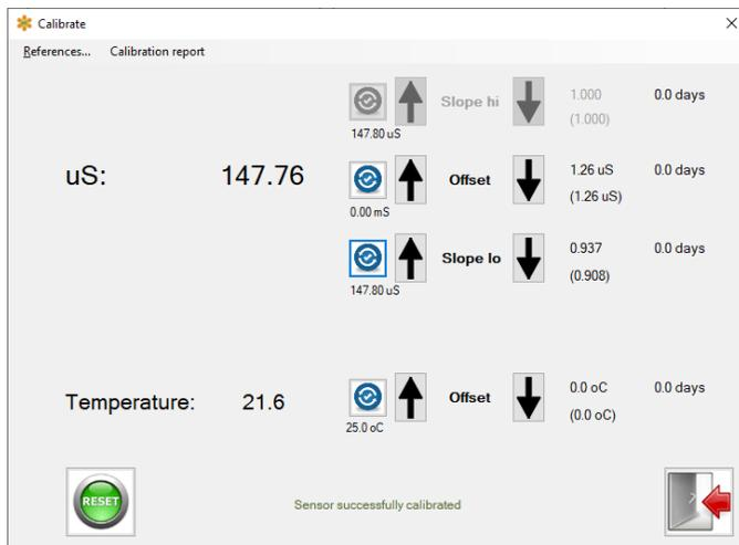
**Step 3 - Perform grab sample slope calibration in-situ if needed**
