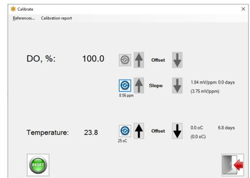
Reading shows 100% saturation in the number of seconds set for dampener & shows the DO ppm used for calibration at current temperature and air pressure.
