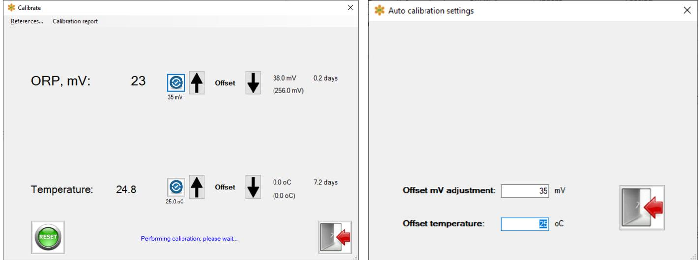
Clicking on the “Calibrate” menu loads screen above when HiQDT-ORP standard or wide-range sensor is connected. The calibrated ORP (mV) and temperature reading is displayed based upon the current calibrations for the connected sensor.
