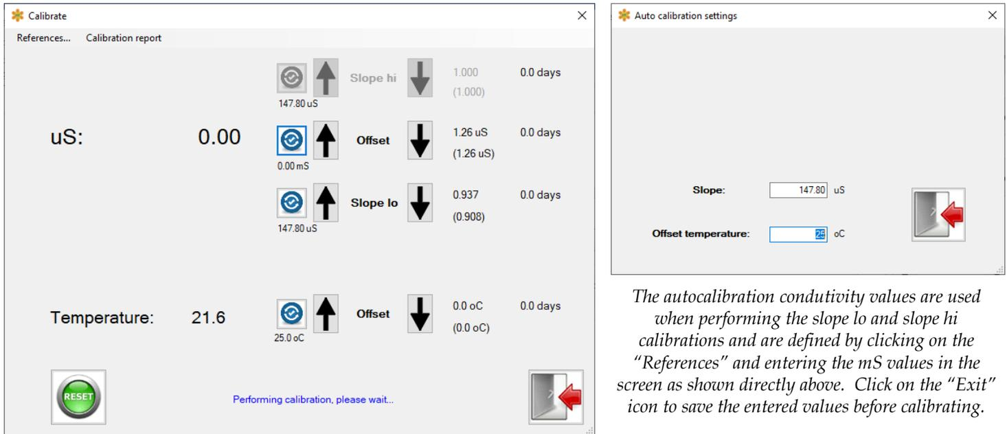
The screenshot displays two windows from the software interface. The 'Calibrate' window on the left shows the following data:
