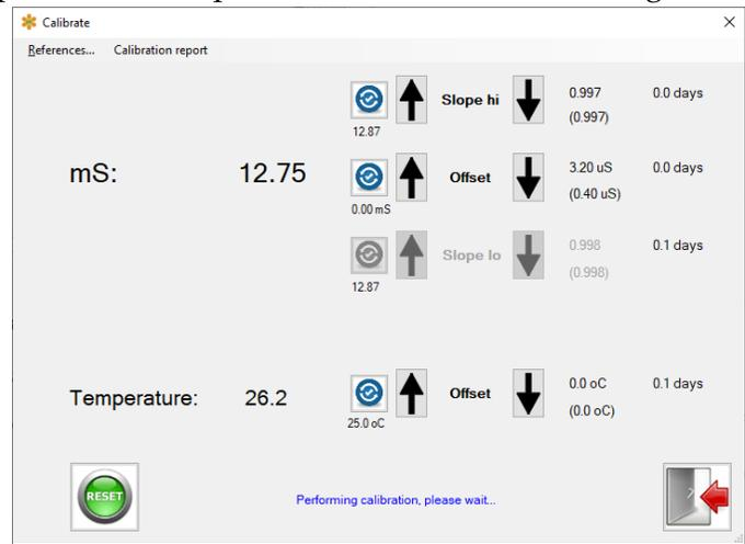
**Step 2 - Perform Slope calibration in range mode to be used**
