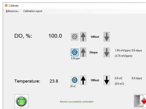
If autoread calibration is completed, “Sensor successfully calibrated” is shown for a period of time as confirmation.
