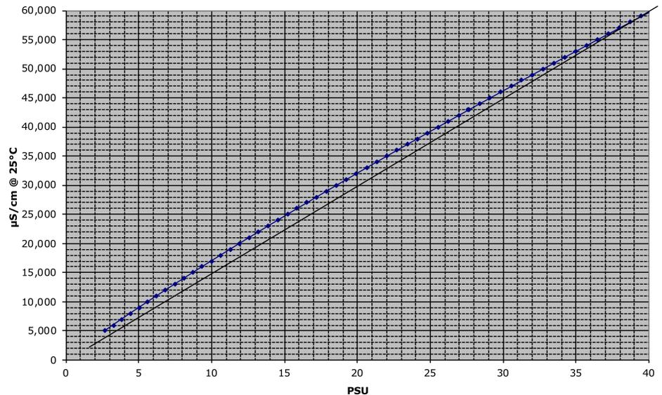
*Salinity computed from the measured conductivity. Curves that define the relationship between measured conductivity and the computed salinity in PSU are preprogrammed into the sensor with a full range of 0.000 to 50.000 PSU.*
