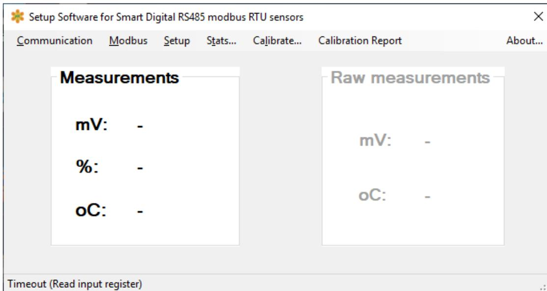
*If no HiQDT sensor is connected there will be dash placeholders for the Calibrated & Temperature Compensated Process Value(s) as well as the raw absolute mV & °C values*
