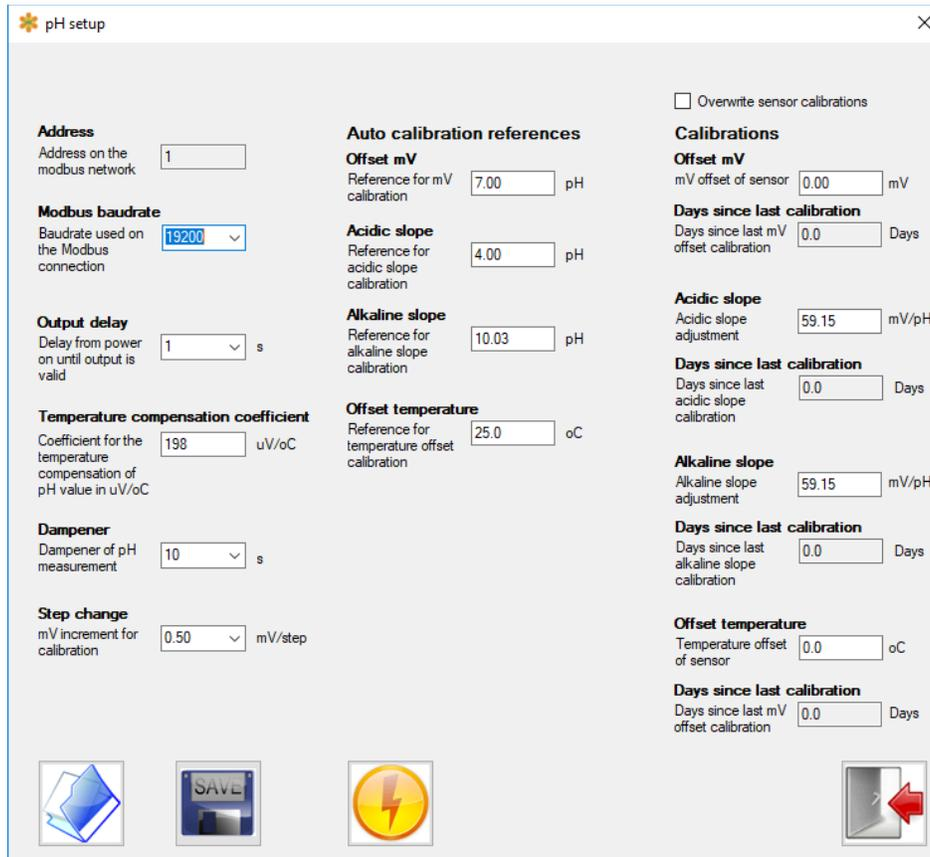
The values for your connected HiQDT sensor may differ from what is shown above depending upon the configuration that was performed at the ASTI factory and/or your local distributor or agent. The assigned value or setting can be modified for any given parameter to an alternate choice within the permissible range or limits at any time as desired.
