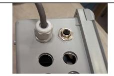
Proper enclosure opening location for M12 cable assembly fitting.
