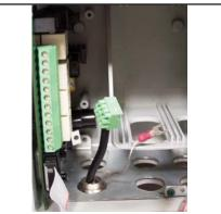
M12 cable assembly wired to 4-lead Profibus terminal block.
