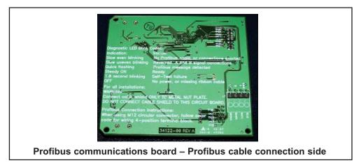
Profibus-configured Model 1056 units also include a pre-installed 10-lead ribbon cable that interfaces the communications board to the main PCB. Upon initial start-up, the Profibus communications board will be recognized by the main PCB microprocessor.
