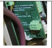
Profibus board showing removable 4-lead terminal block
