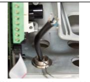
M12 adaptor cable assembly secured to grounding plate.
