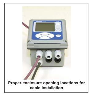
Secure the purple Profibus cable with a cable gland fittings and nut from the outside of the enclosure to ensure a proper seal. Note that the cable gland fittings (PN 23554-00 - Cable Gland Kit, Quantity 5) does not require the securing nut inside the enclosure to properly install the fitting. Simply thread the fitting into the grounding plate inside the enclosure and tighten.
