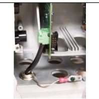
Wired 4-lead terminal block installed on Profibus DP board.
