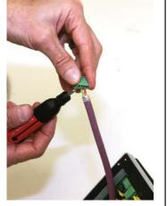
Wiring Profibus cable to 4-lead terminal block
