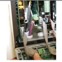
Profibus cable and terminal block installed to Profibus board
