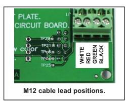
4. Slide the wired 4-lead terminal block onto the 4 pins protruding from Profibus board on the left side.
