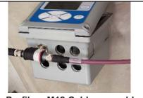
Profibus M12 Cable assembly attached to Profibus network T-cable fitting
