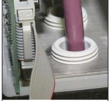
Cable gland fittings secured on internal grounding plate.
