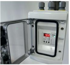
Single Channel Contacting Conductivity Transmitter 3TX-2M-CON-2.0/200-A-PS
