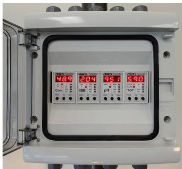
A typical system is shown above with free ammonia (ISE) and pH as inputs for the TOT to compute total ammonia. The 3TX-CON conductivity is the third optional input above but could be a DO, ORP or ISE measurement.
