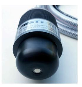
Close-Up of the fully submersible AST-DO-T Galvanic DO sensor with Pt100 TC is above. Optional NPT submersible assembly option is installed in photo of the model shown above. Inline Low-Flow Cell mounting adapters are also available (inquire to factory for details).
