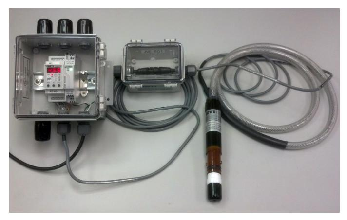
The Q5M (male) quick disconnect termination from the sensor are mated to the Q5F (female) quick disconnect termination for the cable extension inside the 1MF NEMA 4X waterproof J-Box. The sealing cable glands must be well secured to both the 1MF enclosure as well as onto the cables, and the lid must be fastened shut to preserve the NEMA 4X rating.
