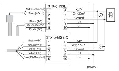
The wiring for sensors with and without preamplifiers are detailed above. Note that these two wiring details represent interface with two altogether different hardware versions which must be selected at time of purchase. Care should be taken to ensure that the proper wiring scheme is used.
